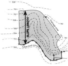
Dispersing Flow: Proper applications of silt fence will allow all the intercepted runoff to pass as diffused flow through the geotextile. Runoff should never overtop silt fence, flow around the ends, or move in any other way as concentrated flow from the practice. If this does occur, maintenance, alternative silt fence layout, or other practices are needed.
