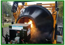
The Service Department recently acquired and trained on a new piece of equipment – KM T-2 Asphalt Recycler. The recycler has a production rate of approximately 4 tons per hour. This will allow the Service Department to have access to hot mix asphalt year
