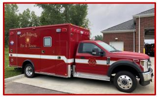
(rear box) is mounted on a Ford F550 four wheel drive chassis and has a liquid spring suspension for increased patient comfort during transport. Some new features that this medic unit will have is an internal negative pressure ventilation sys-
