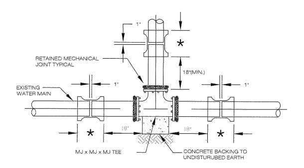
1. \* CONNECTION SHALL BE MADE WITH RETAINED MECHANICAL JOINT SOLID SLEEVES (SHORT OR LONG PATTERN) DUCTILE IRON CLASS 350 OR CAST IRON CLASS 250 OR COMPRESSION COUPLINGS.
