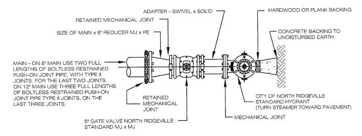
1. IN LIEU OF SWIVEL BRANCH TEES AND ADAPTERS CONTRACTORS MAY FURNISH HYDRANT BRANCHES HAVING RETAINED MECHANICAL JOINTS INCLUDING HYDRANT SHOE. ALL MECHANICAL JOINTS SHALL HAVE FIELD APPLIED ONE (1) COAT OF BITUMASTIC PAINT. ALL MECHANICAL JOINTS SHALL BE POLYETHYLENE WRAPPED IN ACCORDANCE WITH AWWA C-105/A21.5-88 CLASS "C" METHOD "B".
