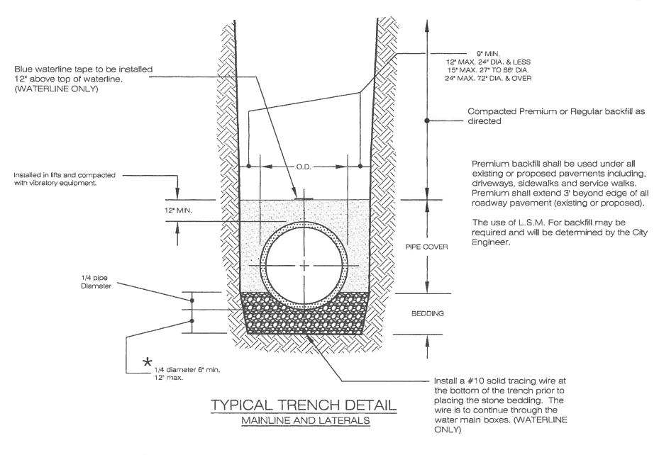
Premium backfill shall consist of course interlocking aggregate O.D.O.T #304 or Low Strength Mortar backfill, Type 2.
