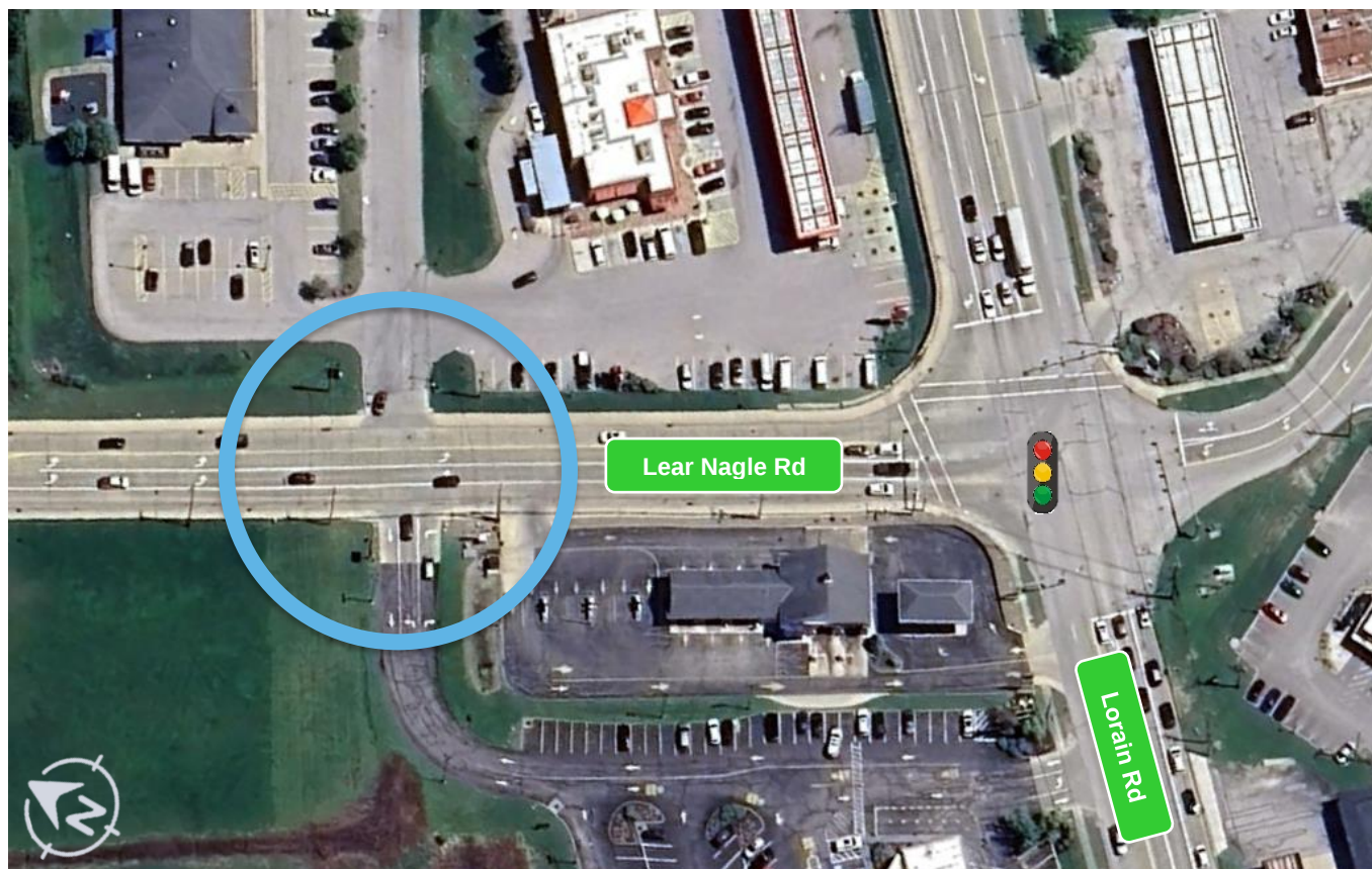
Figure 6 - Access Driveways on Lear Nagle Rd Approaching Lorain Rd
